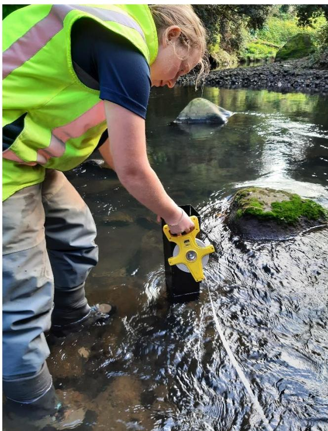
**Photo 4** Monitoring of suspended fine sediment by black disk visual clarity.
