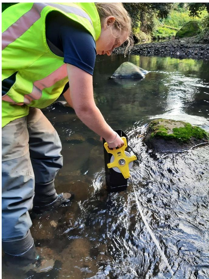
**Photo 2** Monitoring of suspended fine sediment by black disk visual clarity.
